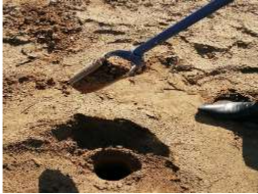
Figure 2: Soil sampling using a hand auger
