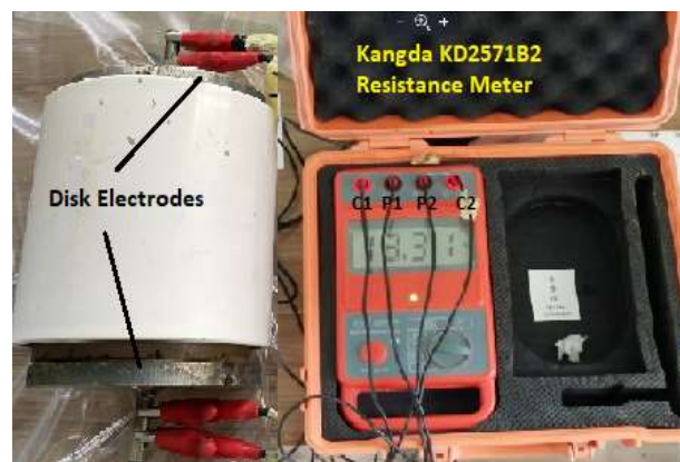
Figure 6: Set up of the ER measurements
