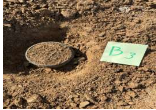
Figure 3: Soil sampling using the core cutter
