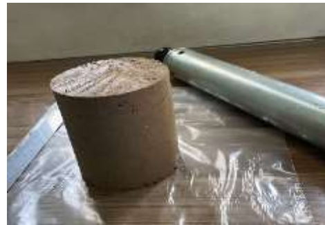
Figure 5: Compacted soil specimen
