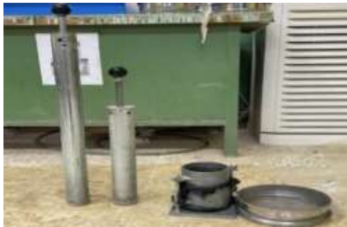
Figure 4: Soil compaction tools
