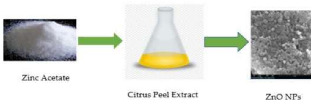
Figure 4: Synthesis of ZnO nanoparticles by Citrus sinensis fruit peels
