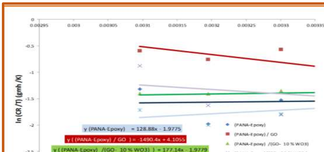
Figure 8-B: Transition state diagram of corrosion of low carbon steel in (1M HCl) in the presence of (GO - 10 % WO 3 / Epoxy-PANA).
