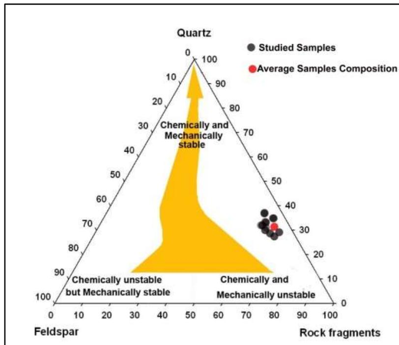
**Figure 8:** Ternary diagram of the stability of the Injana Formation sandstone [19].
